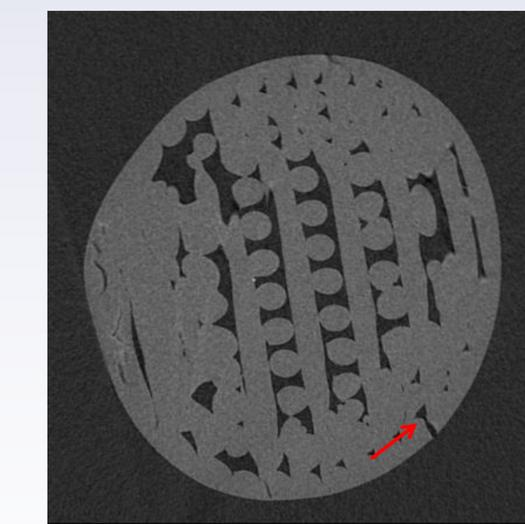
Surface cracks and interior channels are revealed by micro computed tomography. These can occur despite 3D print settings for 100% infill in fused filament prints. Slice by slice examination of 3D Prints (shown above) demonstrate that surface defects can extend beyond exterior shells into the print where they can communicate with longitudinal conduits resulting from incomplete welds or infill.
