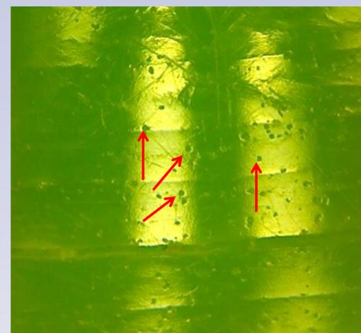
Microporosity on print surface are not necessarily correlated with boundary layers of lamination.
