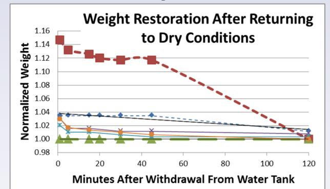
If water enters 3D print, it may be retained for hours. Retained water may serve as a culture medium for microbial growth and subsequent infection of a surgical site or wound underneath the cast/splint.
