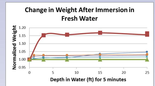
Visually smooth 3D printed casts/splints admitted water ranging from 0% to >15% ± 1% of print dry weight, depending on process controls. With appropriate 3D print technique, waterproofing was maintained for 30 minutes at depths of 25 feet.
