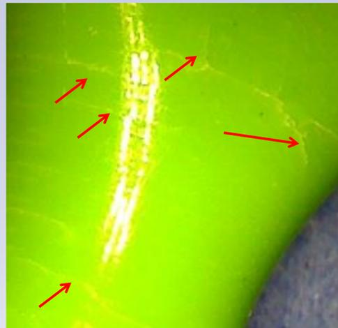
Surface cracks are most frequently aligned with layers of lamination, but may extend across layers.
